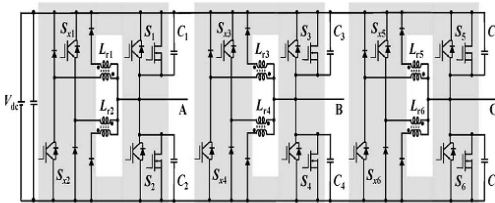
Fig. 3. Circuit Diagram of three-phase soft-switching-module-based inverter.
