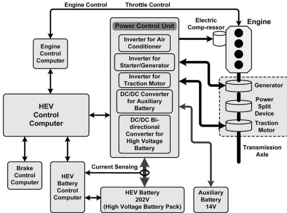
Fig. 2. Power control unit (Toyota Hybrid Synergy II).
