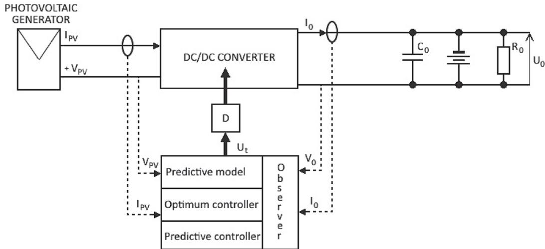
Fig. 3. Photovoltaic station model predictive control block diagram
