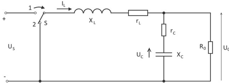
Fig. 5. Lumped parameter model of the buck converter
