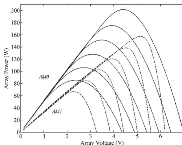
Fig. 1. Array power versus its voltage for the temperature of (from right to left) 273,300, 325,350,375, and 400 K. Solid lines for AM0 (air mass) condition, and dash lines for AM1 condition
