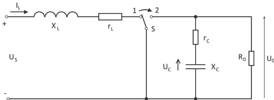
Fig. 4. Lumped parameter model of the boost converter
